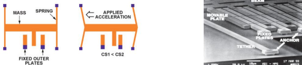
**Figure 1. MEMS accelerometer structure. Figure 2. ADXL50 MEMS accelerometer structure.**
